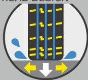
The inside and outside of the tire have a different tread pattern (grooves, void ratio...) to provide maximum grip in very different and variable conditions (wet, damp, dry, even muddy in certain situations).
