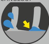
*The tread is specifically developed to break up the water film and prevent aquaplaning. The evacuation grooves are reinforced with deep transverse sipes to break up the film of water.*
