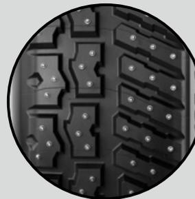
\*Protrusion: length of stud protruding from the tire. The longer the stud protrudes, the better it bites the ice. However, this also increases the risk of tearing or breaking the stud.
